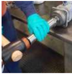
fit shaft with hollow drift
