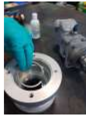
fit O-ring - seat - retainer ring and circlip
