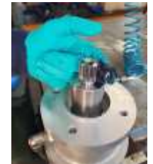
Apply grease to spline
