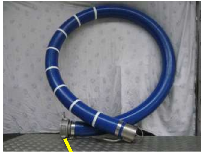
Inlet hose with suction head and ROV manipulator handle.
