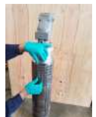
Slide joint section to remove screen from pump
