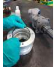
fit O ring into adaptor recess
