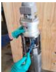
Fasten pump affixing cap screws
