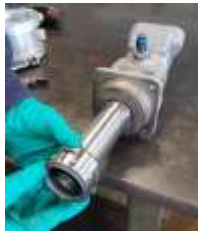
Push seal onto shaft with silicone grease
