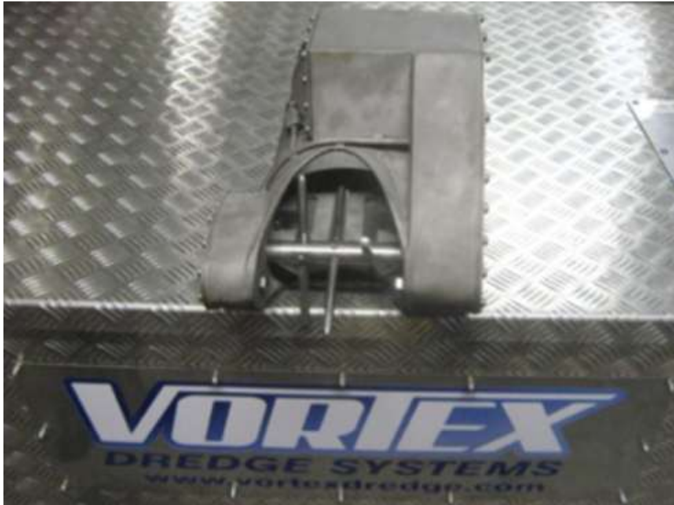
Another option for difficult soils is using the Vortex Marine Rotary Hoe. See images (left) of Marine Rotary Hoe. Sample videos available on our website.
