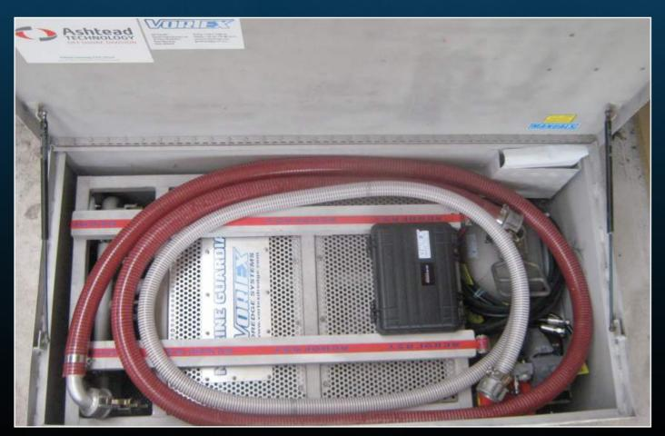
Hydraulic requirement: Pressure = 1500 psi (103 bar) Flow = 5.2 gpm (20 lpm)
