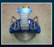
Basic half blade cutter with grab arm mounts and mechanism removed.
