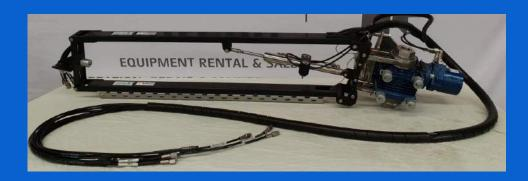
Arm shown here in full 180 degree down position when second stage "knuckle" is functioned allowing exclusive access to underneath asset or fee span.
