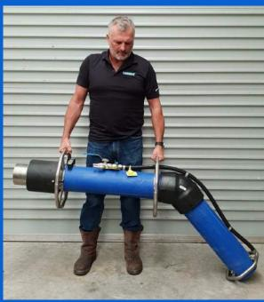
Bolt a bar across the front if dredging or leave open to suck onto large rocks or sand bags to lift away for relocation.
