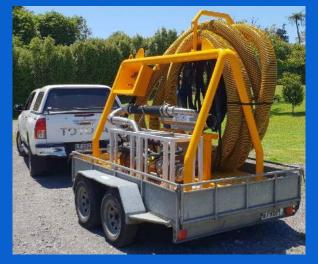
Frame is deployed with 30mtr of suction hose and reversal valve control / jetter hose coiled, connected and ready to go. No need for lowering two loads to seabed. One lift. Easy.
