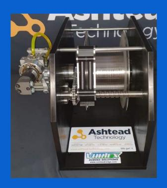
Camera winch designed to be mounted inside or on ROV frame to deploy camera vertically inside hole for visual inspection. Heavy duty and medium duty winches. 4 way and 8 way slip rings. FO slip rings optional
