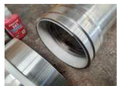
Swivel joint. Remove M8 bolts to disassemble. Do NOT assemble with grease. Assemble dry only. Strip and clean regularly
