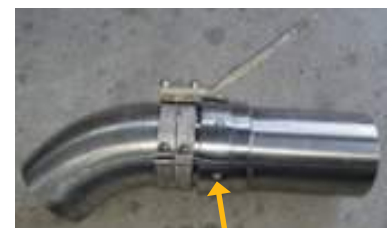
Swivel joint. Remove M8 bolts to disassemble. Do NOT assemble with grease. Assemble dry only. Strip and clean regularly
