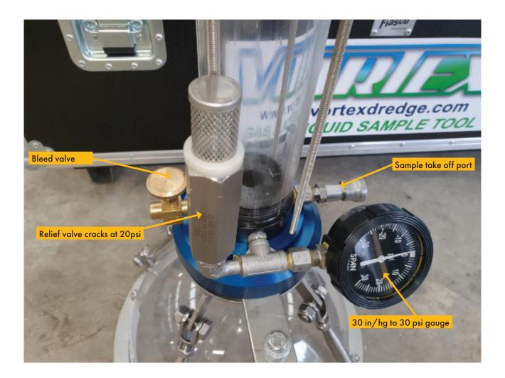
BLEED VALVE IS CLOCKWISE (CW) TO OPEN AND COUNTERCLOCKWISE (CCW) TO CLOSE. DO NOT OVER TIGHTEN.
