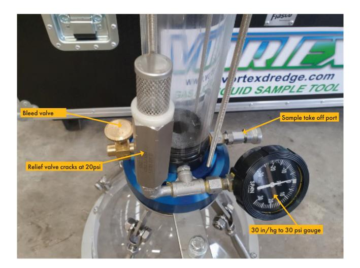
When recovering to deck, ascend as such a rate that the 0 to 30psi pressure gauge does not show over the 20 psi setting of the relief valve.
