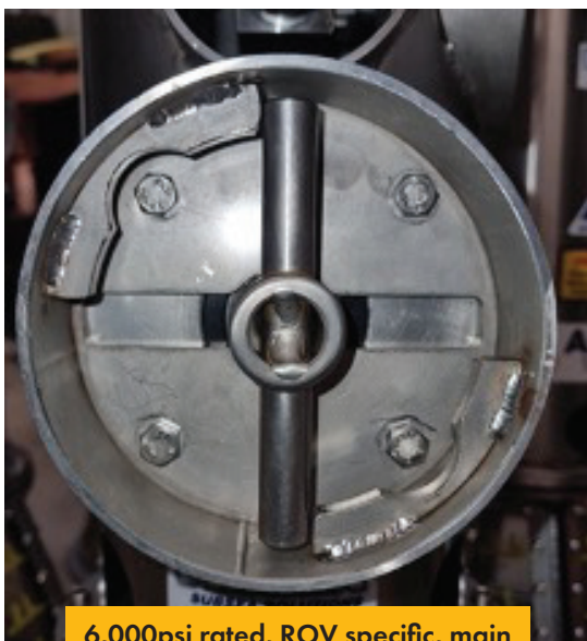
6,000psi rated, ROV specific, main isolation valve and orientation when open
