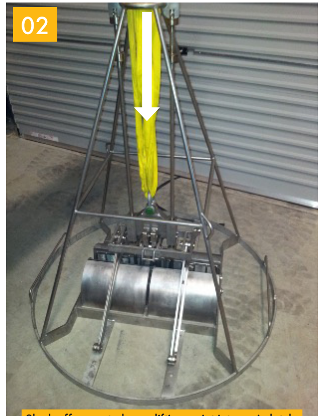
Slack off crane to lower lifting point into main latch.
