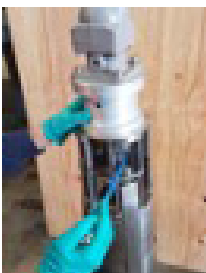
Fasten pump affixing cap screws.
