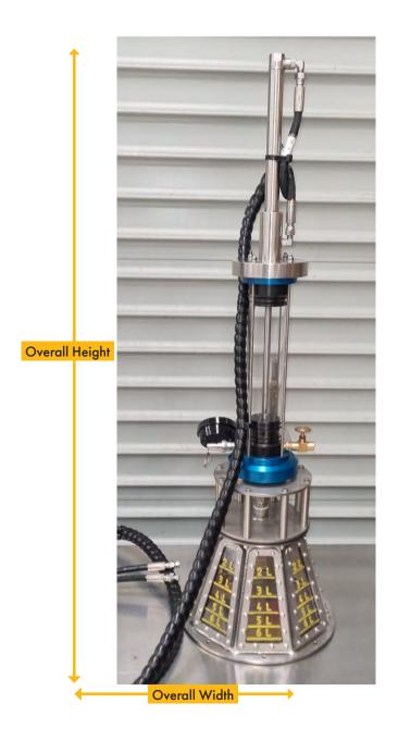
Complete tool weight empty in air = 10kg (22lb) Complete tool dimensions = 940 mm (37inch) overall height / tall  $\times$  460mm (18 inch) overall width.
