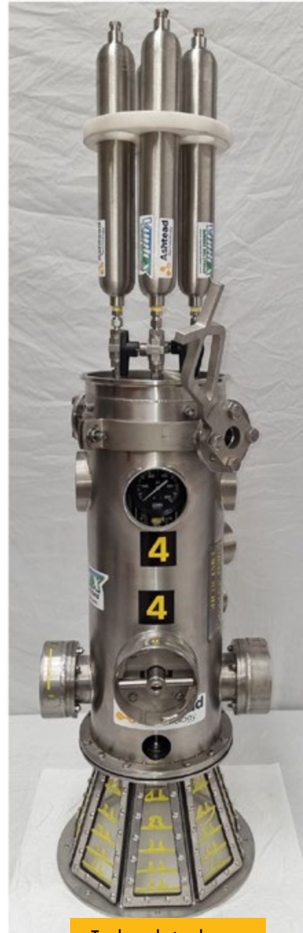
Tool ready to change sample bottles
