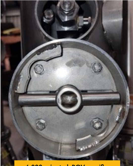
6,000 psi rated, ROV specific, main isolation valve and orientation when closed.
